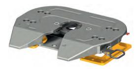
The robust cast steel 36t fifth wheel for heavy duty transport
