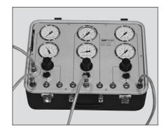
When performing such tests on the road, the brake testing system is placed in the driver's cab.
