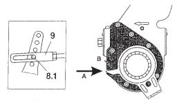
When correctly installed, the Tip of arrow B must match notch A in the control unit.
