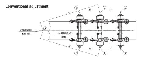
Determine the lengths of the diagonals A - C and A - F for the middle axle (reference axle) by comparison measurements, observing the tolerances.
