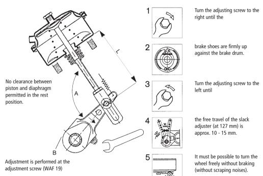
Special instructions apply for automatic slack adjusters (see adjustment procedure on the following pages).
