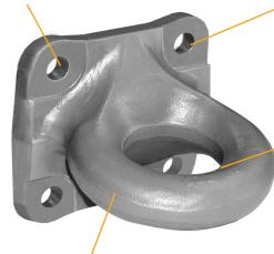
41.4mm diameter cross section. It is induction hardened in the pintle hook contact area for increased strength and wear resistance.
