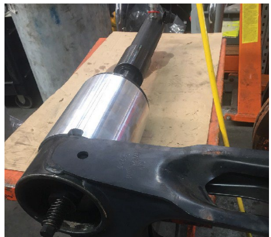
Fig. 7 - Removal tool installation
