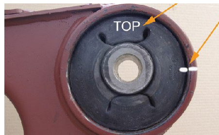
Fig. 15 - Checking installation position
