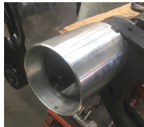
Fig. 12 - Correct receiver tube position
