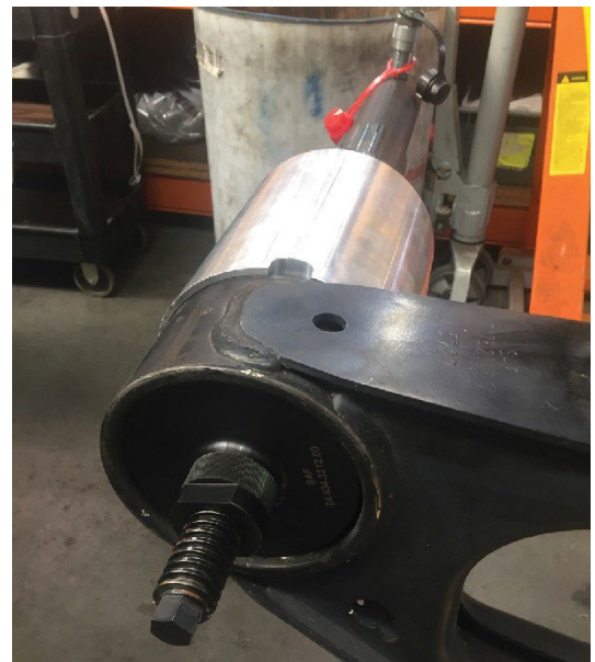
Fig. 6 - Removal tool installation
