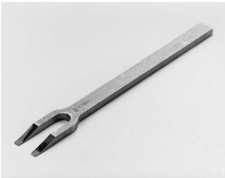
6. Wedge fork for tappet with boot SAF Part No. 4 434 1065 00
