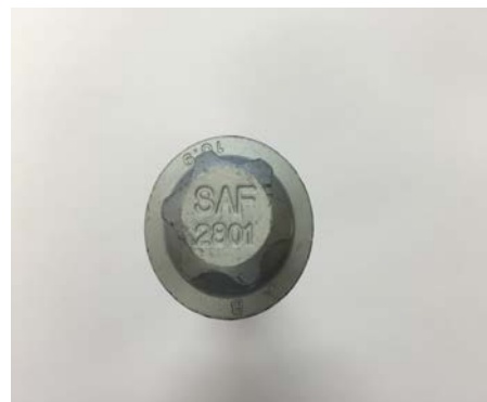
SAF marking on the original SAF- Hexagon screw including part number 2801. The screw head also states the manufacturing category (10.9) on the screw head
