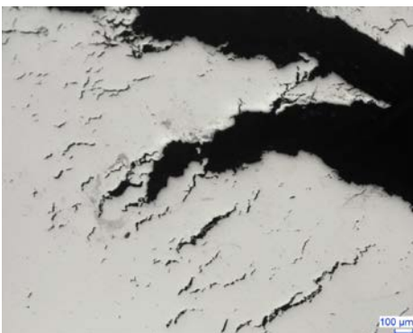
Microscopic cracks around the screw head of the replica Hexagon screw.
