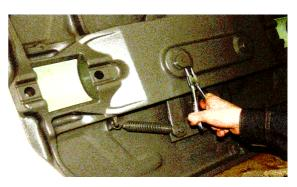
6. Remove the bolt from the coupler jaw.
