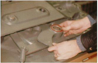
Attach all three tension springs on the coupler jaw and the unlocking handle. Pull the unlocking handle outwards and set the locking mechanism in the coupling position.
