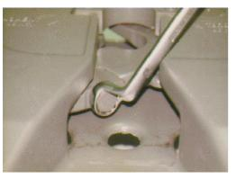
The adjustment must be carried out with a **new** kingpin.
