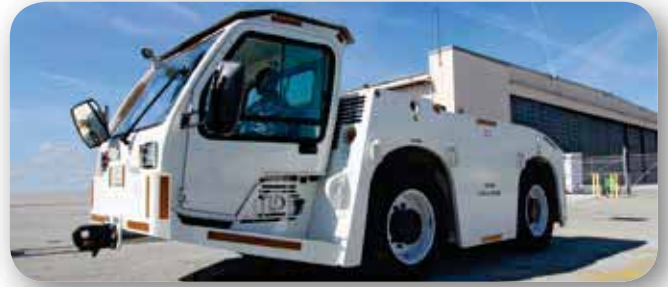
TLD Large Land Based Tow Tractor (LLTT) for U.S. Navy (2011) with HOLLAND CP-360-S01340 Couplers
