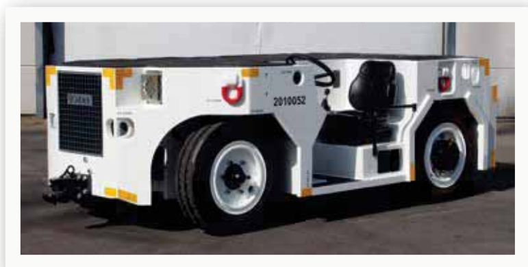
Schopf Shipboard Tow Tractor (STT) for U.S. Navy (2013) with HOLLAND CP-400-GSE Couplers
