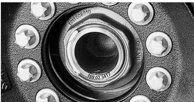
Identification of axles in case of type plate absence Serial No. on spindle end, Rh side.
