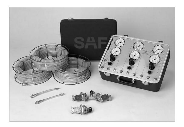
The SAF brake testing system is required for adjusting and testing air brake systems on vehicles and for overcoming problems related to the balancing of air brake systems between tractor and trailer or semi-trailer.
