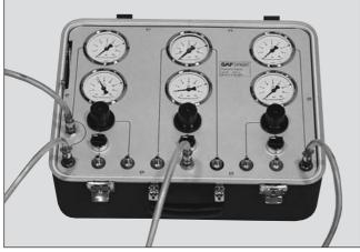
The pressure set at the middle precision control valve (02) is displayed on pressure gauge (6). This brake pressure can be admitted to the trailer brake line via port 6 by actuating the switching valve and actuates the brakes of the trailer.
