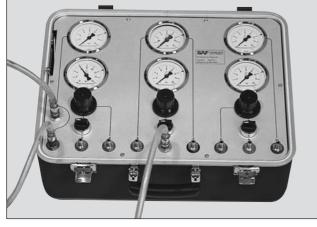
Connect the test port "Output LSV controller" to port 10 of the brake testing system.
