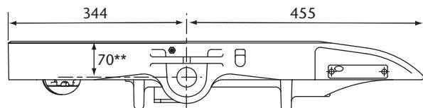
\*\* Bracket pin centre line to top surface
