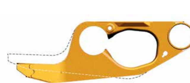
More offset: The new functional suspension arm allows low ride heights
