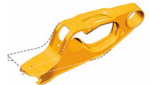
Designed asymmetrically: The spring offset ensures freedom of choice in terms of tyres
