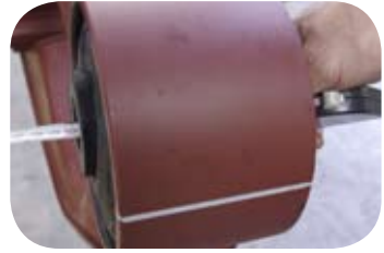
Fig. 13 · Checking the spring center
