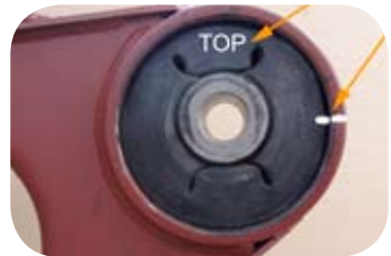
Fig. 14 · Checking the installation position
