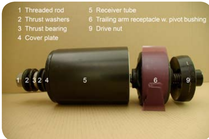
Fig. 1 · Identification of removal tool components
