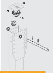
**BEVEL AND PINION GEAR**
