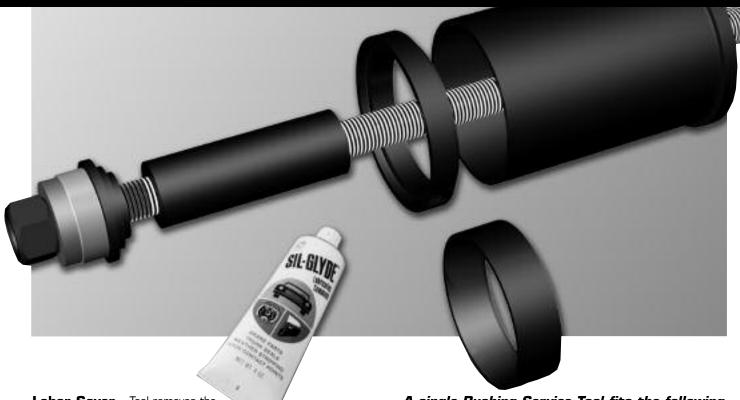
**Labor Saver** – Tool removes the worn-out front pivot bushing and installs the new bushing. The equalizing beam does not have to be removed from the axle connection.
