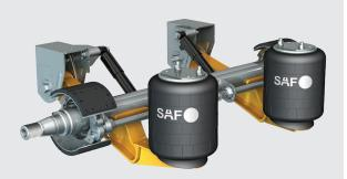
For low profile trailer applications that require 17.5" and 19.5" wheel sizes, the SAF CBu and CBy suspension models accommodate 12.25" x 7.5" drum brake packages. The CB models feature industry standard tapered spindles. Optional parallel spindles also available.
