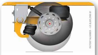
The patented Auto-PosiLift<sup>™</sup> feature automatically lifts the front axle when the system senses that only one axle is necessary to carry the load.
