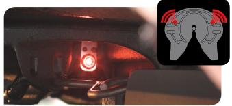
**FAILED COUPLING** – In the case of a failed coupling attempt, bright red flashing LED lights assist the driver to quickly recognize a potentially costly mistake before attempting a tug test or driving away.
