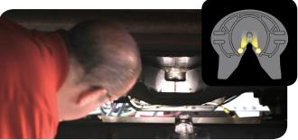
**SUCCESSFUL COUPLING** – A successful couple triggers highintensity white LED lights, strategically aimed at the kingpin and lock for enhanced visibility during the inspection process, especially in poor weather and low-light conditions.
