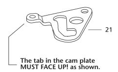
3. Position the cam plate attachment hole over the proper casting lug hole, as shown.
