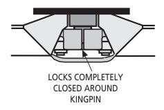
2. Check for resistance between the locks and lock tester one final time, adjust as needed.
