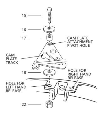
4. Slide a 1-3/4" washer (*Item 16*) between the cam plate and casting lug hole with the rounded side of the washer facing the cam plate.
