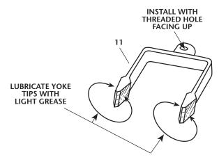
2. With the threaded hole facing up, slide yoke (*Item 11*) into casting. Tap lightly to seat yoke around locks.
