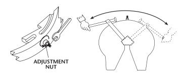
The fifth wheel is properly adjusted when there is resistance between the locks and the lock tester, but the lock tester can still be rotated by hand, as shown.
