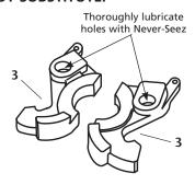
2. Align the lock jaws (*Item 3*) in the casting, as shown.
