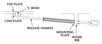
2. Bolt the mounting plate (attached to the handle) to the hole in the casting top plate using the 1/2" x 1-3/4" long bolt, 1/2" washer, and 1/2" locknut (see below.) Be sure to attach the plate to the inside of the of the "inside" rib on the casting, and that the 1/2" washer is on the headed end of the bolt.
