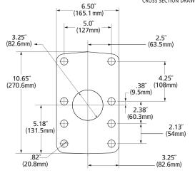
The PH-405 can be used with or without air chamber and is compatible with drawbar eye dimensions of 2.375" (60mm) I.D. with a 1.63" (41mm) cross section.
