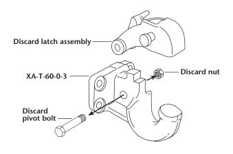
Apply Never-Seez® to entire shaft of the new pivot bolt (not on threads).
