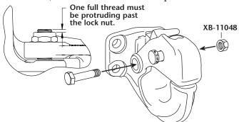
**WARNING**DO NOT reinstall a removed lock nut. Always install a new lock nut when removing or replacing latch assembly. A reinstalled nut may not retain properly and could result in an unintended trailer separation.
