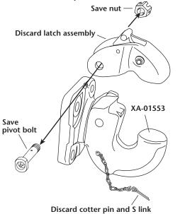
2. Clean and grease the ports in the old pivot bolt. Apply Never-Seez<sup>®</sup> to the entire shaft of the pivot bolt (not on threads).
