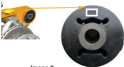
Image 2: Follow the "TOP" label for installation position
