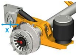
Image 1: Joint elasticity: x = \pm 14 mm, 28 mm total
