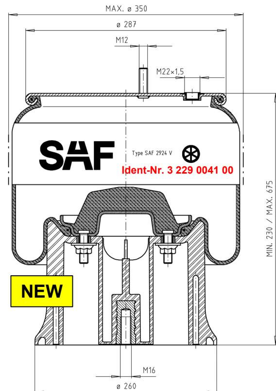
**NEW** > SAF 2924V has a piston with an integrated thread for fixing on the suspension arm with a hex bolt.
