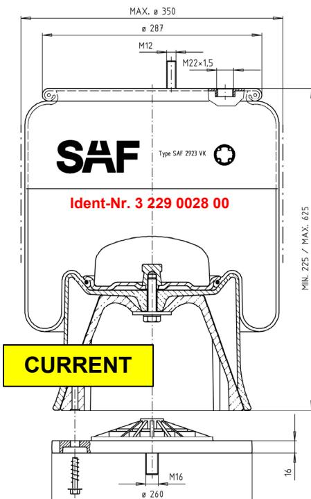
The main difference between the current and the new air spring is the new piston design and the much easier installation on the INTRA suspension arm.
