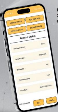
In addition to the warning message on the dashboard in the cab, SAF TIRE PILOT I.Q. offers detailed evaluations of the system via an app and WiFi.
