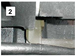
4. After correctly adjusting the play, mark the closed position for the snap hook on the locking handle.
