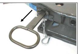
2. The semitrailer plate must be approx. 5 cm lower than the fifth wheel coupler plate. Reverse with the tractor slowly under the semitrailer. The locking mechanism engages automatically.
