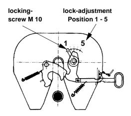
Loosen the fillister screw M10 SW 8 on the fork so that the fork can be moved. The regulation by one notch is equal to an adjustment of 0,5 mm. Re-tighten the screw with a torque of 46 Nm.
