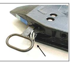
ATTENTION: In any case, it must be made sure that the Fifth wheel is properly locked and secured.
