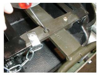
5. Pull out the locking handle and file out the marked area.
