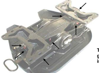
The rocker assembly is equipped with 9 grease nipples, each of which, must be individually greased.
