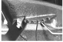
If this is not possible, return fork by one or more notches. If no further adjustment is possible, both coupler jaw and wearing ring must be replaced (see "Wear limits").
