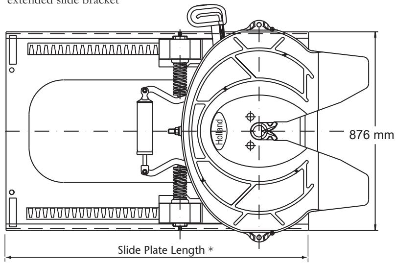
FW3510 top plate on 194 / 219mm high slide brackets with air cylinder under top plate
