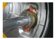
Outer S-camshaft compact bearing
