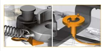
The Safety Sensor System for the SK-S 36.20 fifth wheel REmote COntrolled Safety System
