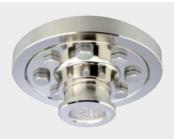
D-value: 320 kN Semi-trailer skid-plate thickness: 16 mm Approval mark: E1 55R-01 2426
