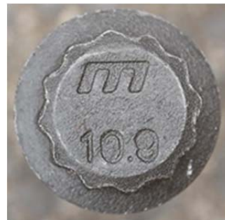
replica bolt with lower grade 10.9
