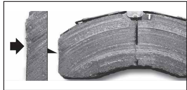
5.1.1 - Brake pad with permissibly small cavities
