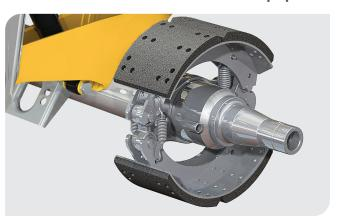
The SAF CBX40 AeroBeam standard configuration features SAF X-Series 5¾" diameter axles with 16½" x 7" extended life brake linings, short cams, and industry standard taper spindles.
