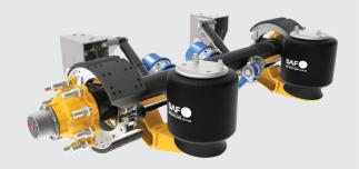
For low profile trailer applications that require 17.5" and 19.5" wheel sizes, the SAF CBu and CBy suspension models accommodate 12.25" x 7.5" drum brake packages. The CB models feature industry standard tapered spindles. Optional parallel spindles also available.
