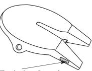
The aluminum Part and Serial No. Tag is located in the same place on all four Yard Spotter Top Plates
