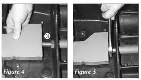
**3.** Position spacer tubes over threaded holes in casting. These spacers come in two different lengths, so be sure to place shorter spacer on the raised portion of casting (Figure 6) (Items 4 &5).
