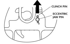
**14.** Securely lift fifth wheel up on edge, allowing for removal of eccentric pin. Reach under the fifth wheel plate to catch the eccentric jaw pin while tapping the base of the jaw pin.
