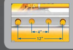
SLOA1480 Upper Body Slider Rails with 4" pin spacing increments for 1-5/8" diameter pins: provide fleets flexibility when positioning their suspension sliders.
