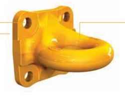
The drawbar eye is 76 mm I.D. with a 41.4 mm diameter cross section. The eye shape is designed to match HOLLAND pintle horns or coupler jaws to assure minimal wear.
