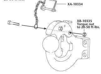
4. Check the latch for proper operation. When closed, the lock must be fully down. Install the D-ring into the hole in the side of the latch, as shown. Snap the spring over the D-ring and pin to secure.
