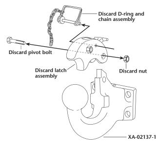
2. Apply Never-Seez<sup>®</sup> to entire shaft of the new pivot bolt (not on threads).
