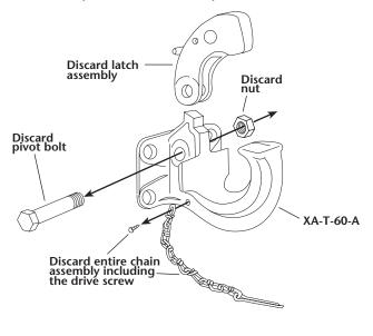
Apply Never-Seez® to entire shaft of the new pivot bolt (not on threads).
