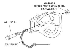
4. Check the latch for proper operation. When closed, the lock must be fully down. Install the cotter pin into the hole in the side of the latch, as shown. Spread the cotter pin to secure it in the latch.
