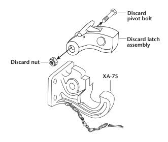
2. Apply Never-Seez® to entire shaft of the new pivot bolt (not on threads).
