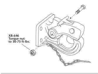
4. Check the latch for proper operation. When closed, the lock must be fully down. Install the cotter pin into the hole in the side of the latch, as shown. Spread the cotter pin to secure it in the latch.
