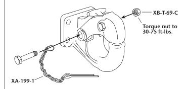
4. Check the latch for proper operation. When closed, the lock must be fully down. Install the cotter pin into the hole in the side of the latch, as shown. Spread the cotter pin to secure it in the latch.
