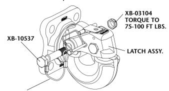
XB-S10647 PIN AND LANYARD: INSTALL LANYARD LOOP SUCH THAT IT IS ORIENTED WITH BOLT HEAD (AS PICTURED)
