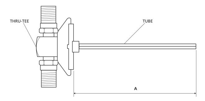
**NOTE:** SAF-HOLLAND provides a "prepped" axle for MTIS (PSI) installation; however, the "Thru-Tee" fittings and other system hardware are ordered separately by the trailer OEM.
