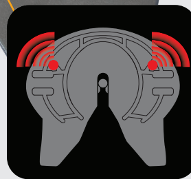
FAILED MODE Red Flashing Warning Lights
