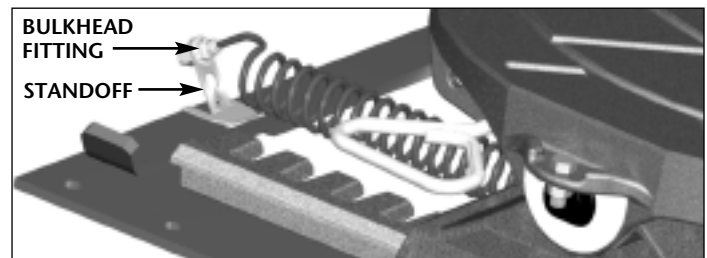
FIGURE 2 Connecting Air Line to the Bulkhead Fitting
