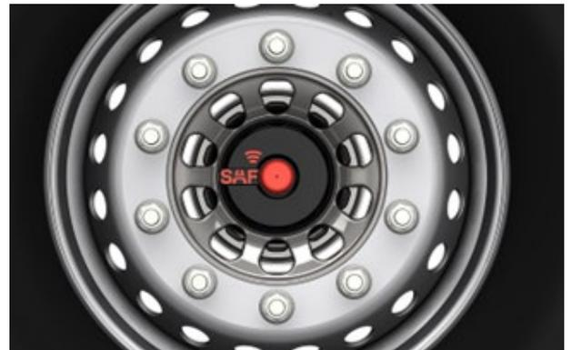
The SAF axles with the NFC chip can be recognized by the red radio symbol on the hub cap.
