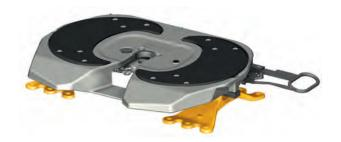
Imposed load: 20,000 kg (2") D-value: 152 kN Overall heights: 128\*, 150, 185, 225, 250 mm ECE test no.: E1 55R-01 0218
