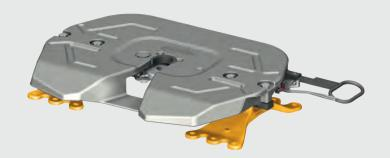
All of the fifth wheels in the SK-S 36.20 range from HOLLAND are particularly light thanks to their design and the use of spheroidal graphite cast iron, and are equipped with a safety latch that allows coupling or uncoupling with one hand.
