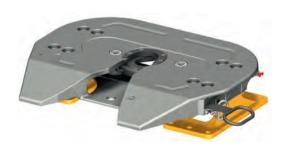
Imposed load: 23,000 kg (2"), 36,000 kg (3.5") **D-value:** 162 kN (2"), 260 kN (3.5") Overall heights: 150, 190 mm ECE test no.: E11 55R-01 8550 (2"), E11 55R-01 8549 (3.5")
