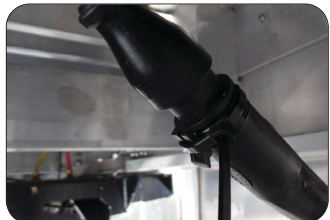
18. Run the wires for the trailer mounted warning light through the trailer crossmembers. Use cable ties to secure the wiring (**Figure 22**).
