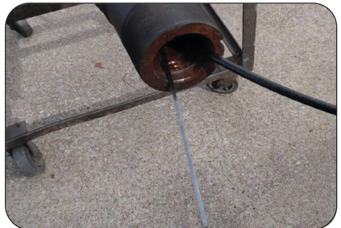
4. Insert 1/4" DOT tubing through from the curbside to the roadside spindle. Leave approximately 6" of air line outside of both spindles (**Figure 8**).
